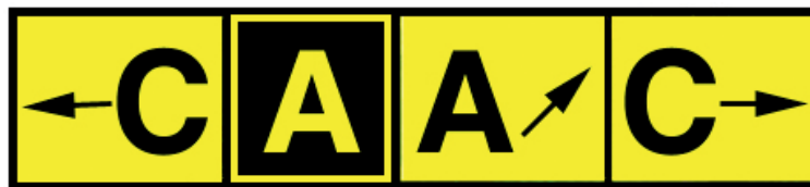
Taxiway Direction Sign combined with a Taxiway Location Sign You are located on taxiway Alpha Nearing taxiway Charlie Taxiway Alpha bears right ahead (dog leg right)
